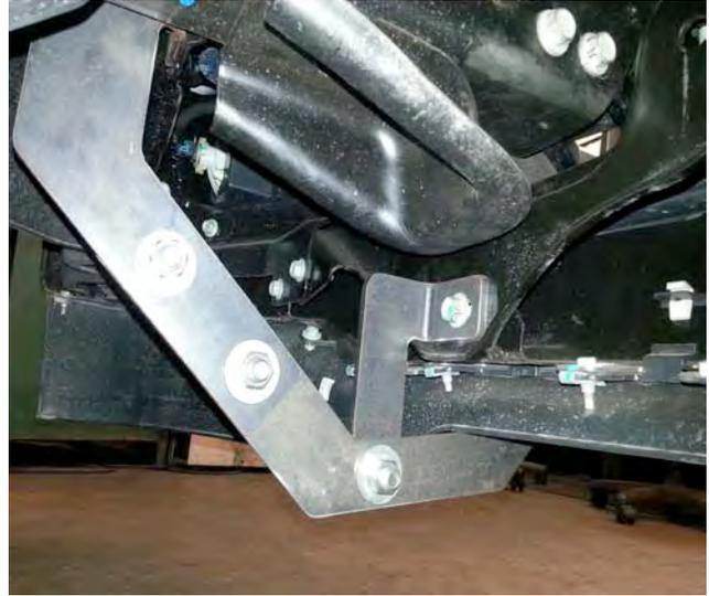
6. Install the grill guard to the mounting brackets by using four black carriage bolts. Level and tighten bolts. Line up the hole of the bottom mounting bracket with the bottom hole in the grill guard. Install another black carriage bolt and tighten. *See photo*
