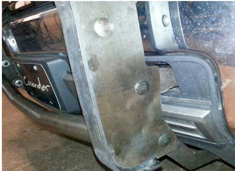
7. On models with sensors, make sure the grill guard (GGC14HBLS) is in the up position of the slotted hole of the uprights. Once installed, check to see if the park assist sensors don't go off. Adjust as needed.
