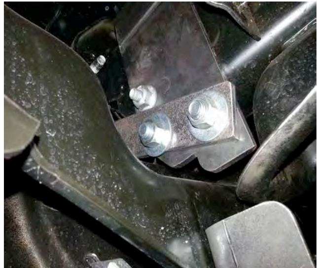
3. Remove the inner bolt (the one closest to the frame) of the bumper side support bracket. Mount the bottom formed bracket parallel to the frame then reinstall the factory bolt. *See photo*
