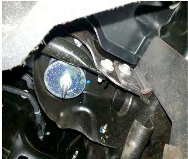
4. Install the bottom mounting bracket to the formed bracket by using two ½” x 1 ½” bolts. Allow a little movement.
