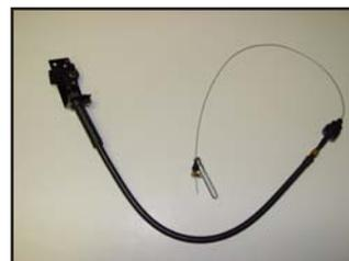
Universal Cable with TPS mounted on Bracket
